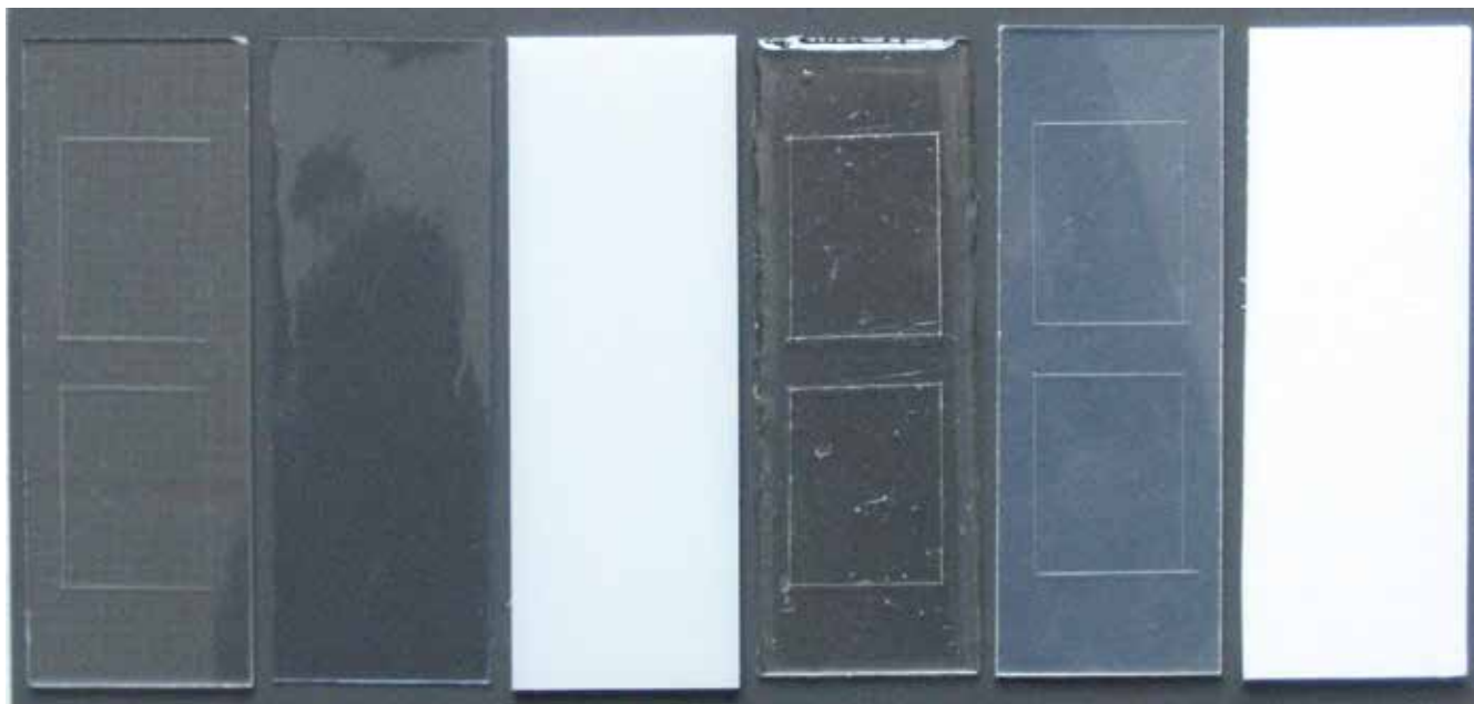
Figure 1. A selection of model plastics. From left to right; polymethylmethacrylate, plasticised PVC, unsaturated polyester (replaced with cellulose acetate), high density polyethylene, high impact polystyrene and expanded polystyrene (only included in the first stage). (photograph by Kathrine Segel).
