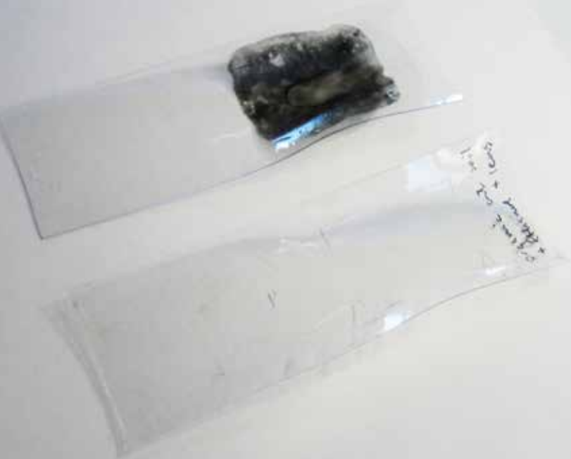
Figure 5. Plasticised PVC model plastics deformed one week after applying organic oil soil (upper). The deformation persisted despite cleaning (lower) (photograph by Kathrine Segel).
