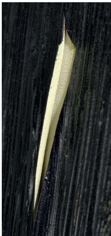
Figure 4. Detail of point of delamination in normal light. Photo: National Museum, Børre Høstland.
