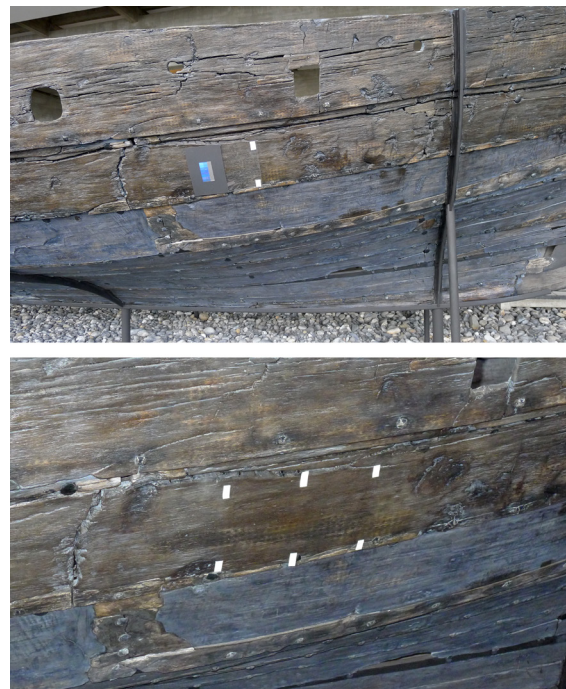
Figure 5. A lightproof plate and a UV filter foil mounted on the side of Skuldelev 3, directly facing the window (top). At the bottom the two areas are shown after the covers were removed after 258 days. The white pads indicates the corners of each cover. The plank on which the covers were mounted was newly cleaned, while the bluish planks below were uncleaned. Photo: Morten Ryhl-Svendesen.
