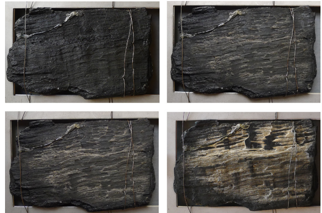
Figure 7. The wood sample exposed to the accelerated light aging test: Before exposure (top left); after 9.5 Mlux-hours (top right); after 15 Mlux-hours (bottom left); and after 43 Mlux-hours (bottom right). Photo: Morten Ryhl-Svendsten.
