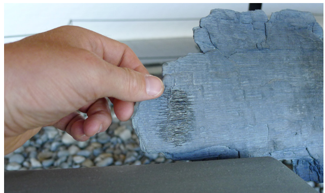
Figure 3. Close-up of a ship plank with the powdery surface, which easily can be rubbed off. Photo: Morten Ryhl-Svendsen.
