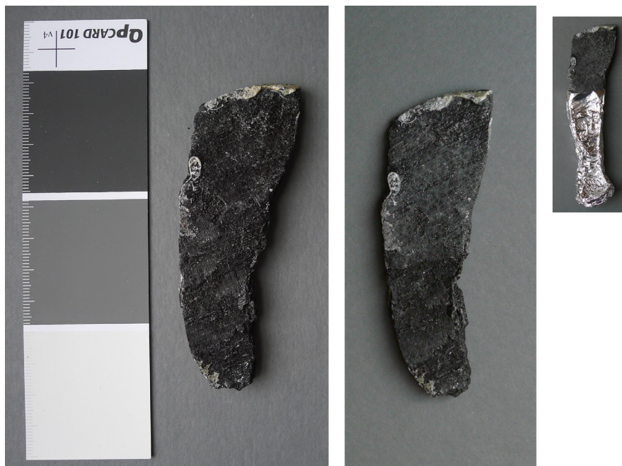
Figure 8. The sample for the UV test, before (left) and after exposure (right). The upper half was exposed during the test and developed a faint white surface, while the lower half was covered by lightproof aluminum foil (see insert upper right). Photo: Morten Ryhl-Svendsten.
